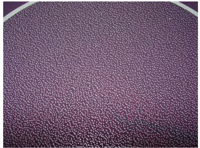
Photo #71 – View of cooktop after 11.68-lb was applied to the dry surface.
