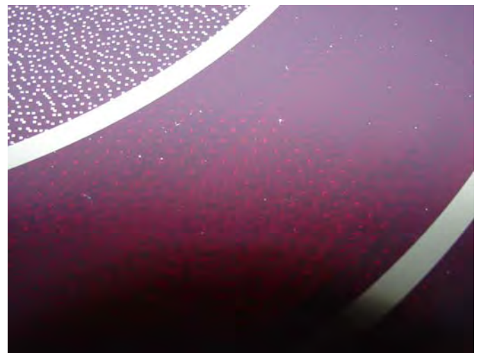
Photo #77 – View of cooktop after 12.48-lb was applied to the wet surface.
