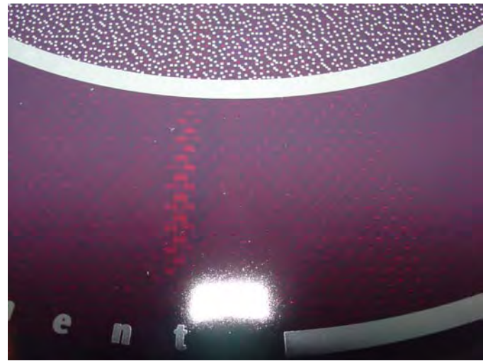
Photo #35 – View of cooktop after 4.48-lb was applied to the dry surface.
