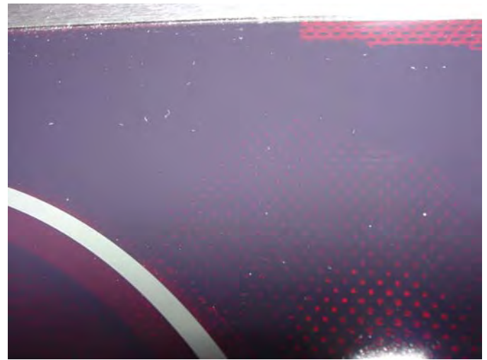
Photo #79 – View of cooktop after 13.28-lb was applied to the dry surface.
