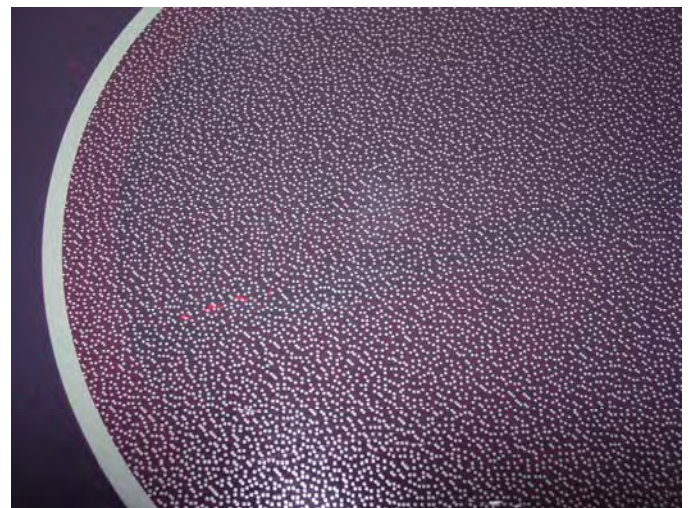
Photo #57 – View of cooktop after 8.48-lb was applied to the wet surface.
