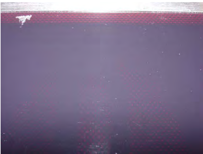
Photo #40 – View of cooktop before 5.28-lb was applied to the wet surface.
