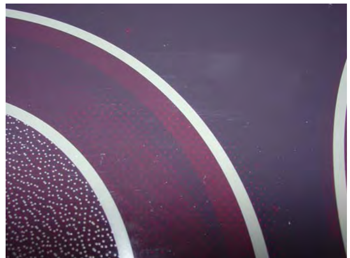
Photo #61 – View of cooktop after 9.28-lb was applied to the wet surface.
