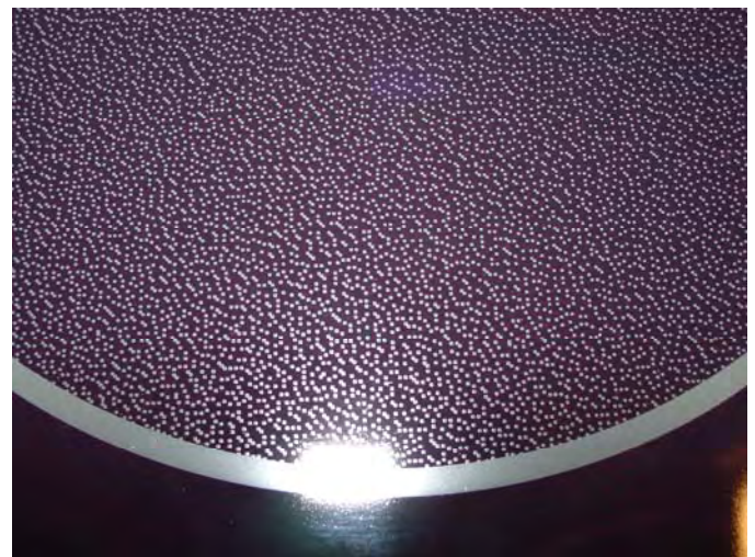
Photo #73 – View of cooktop after 11.68-lb was applied to the wet surface.
