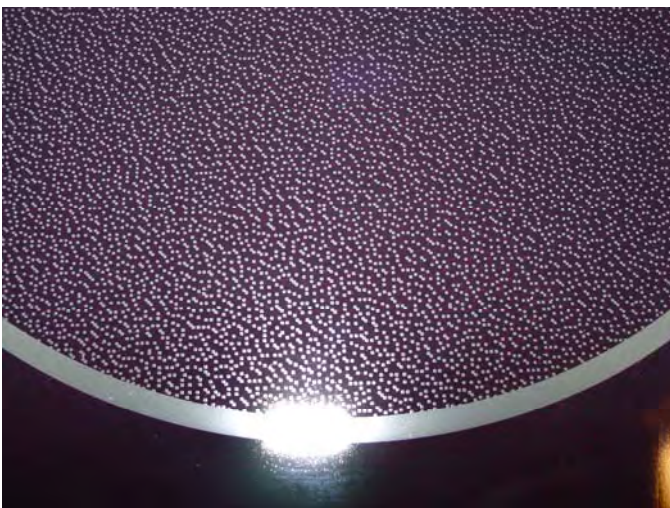
Photo #72 – View of cooktop before 11.68-lb was applied to the wet surface.
