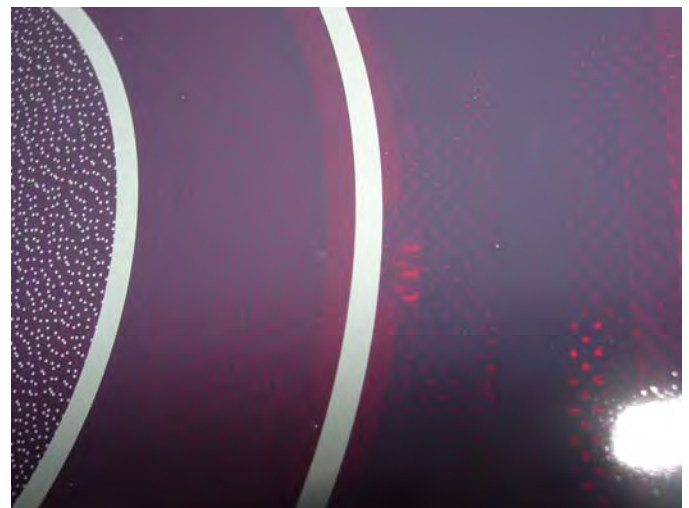
Photo #81 – View of cooktop after 13.28-lb was applied to the wet surface.
