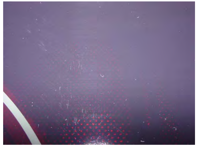
Photo #43 – View of cooktop after 6.08-lb was applied to the dry surface.
