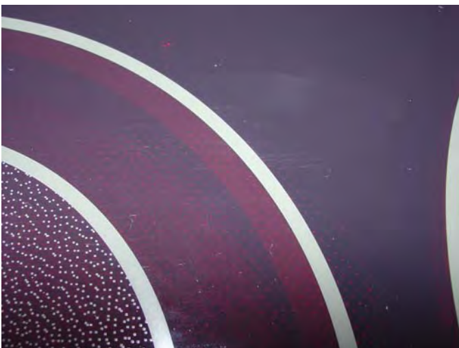
Photo #60 – View of cooktop before 9.28-lb was applied to the wet surface.
