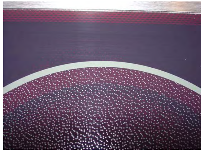
Photo #55 – View of cooktop after 8.48-lb was applied to the dry surface.
