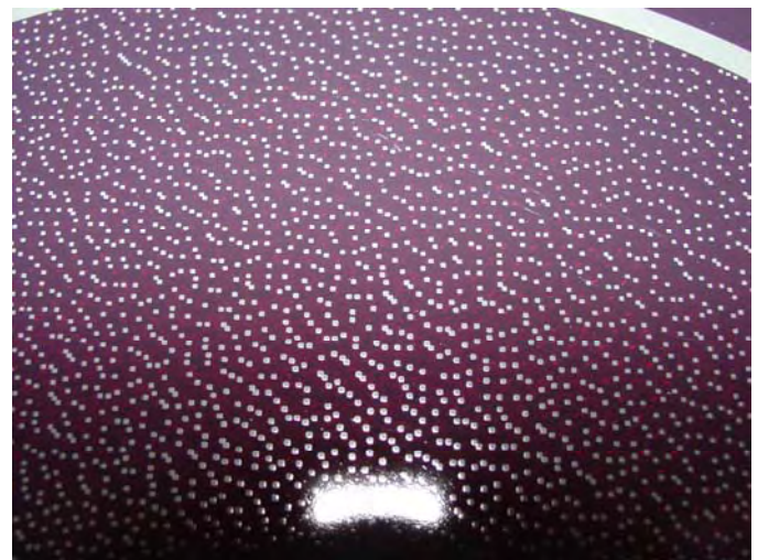
Photo #33 – View of cooktop after 3.68-lb was applied to the wet surface.
